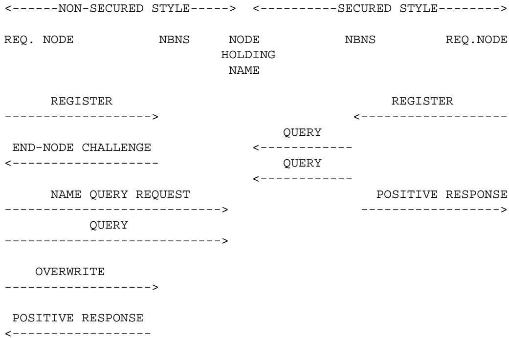
Due to the potential time for the secured NBNS to make the challenge(s), it is likely that a WACK will be sent by the NBNS to the registrant.
