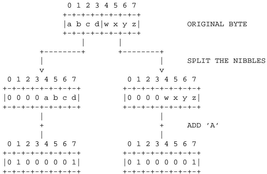
This encoding results in a NetBIOS name being represented as a sequence of 32 ASCII, upper-case characters from the set {A,B,C...N,O,P}.
