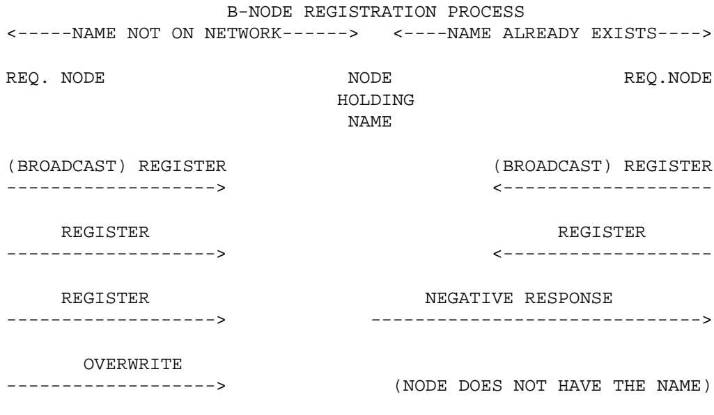
The NAME REGISTRATION REQUEST, like any request, must be repeated if no response is received within BCAST\_REQ\_RETRY\_TIMEOUT. Transmission of the request is attempted BCAST\_REQ\_RETRY\_COUNT times.
