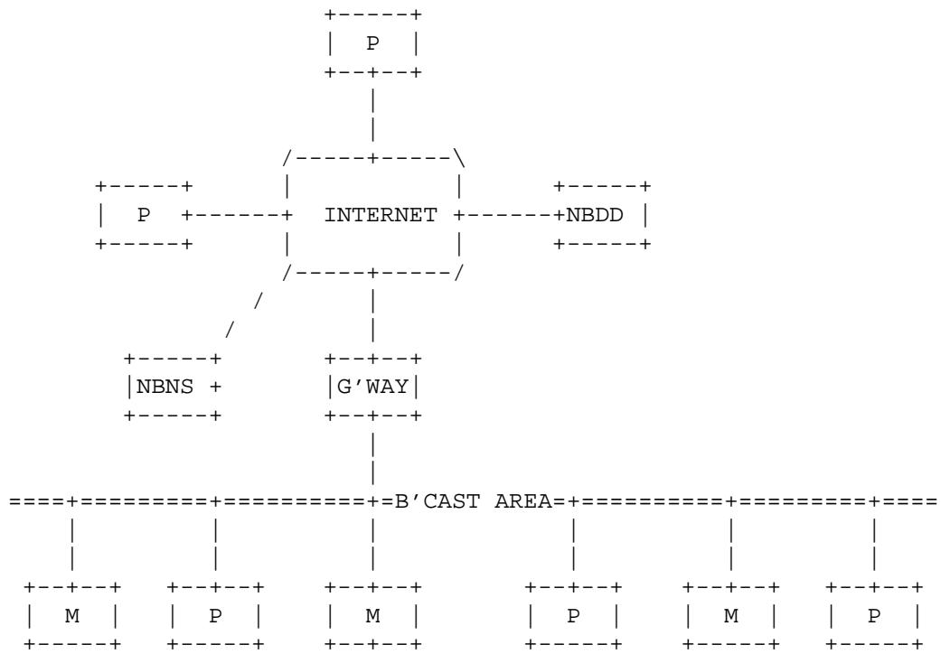
NOTE: B and M nodes should not be intermixed in an internet environment. Doing so would allow undetected NetBIOS name conflicts to arise and cause unpredictable behavior.
