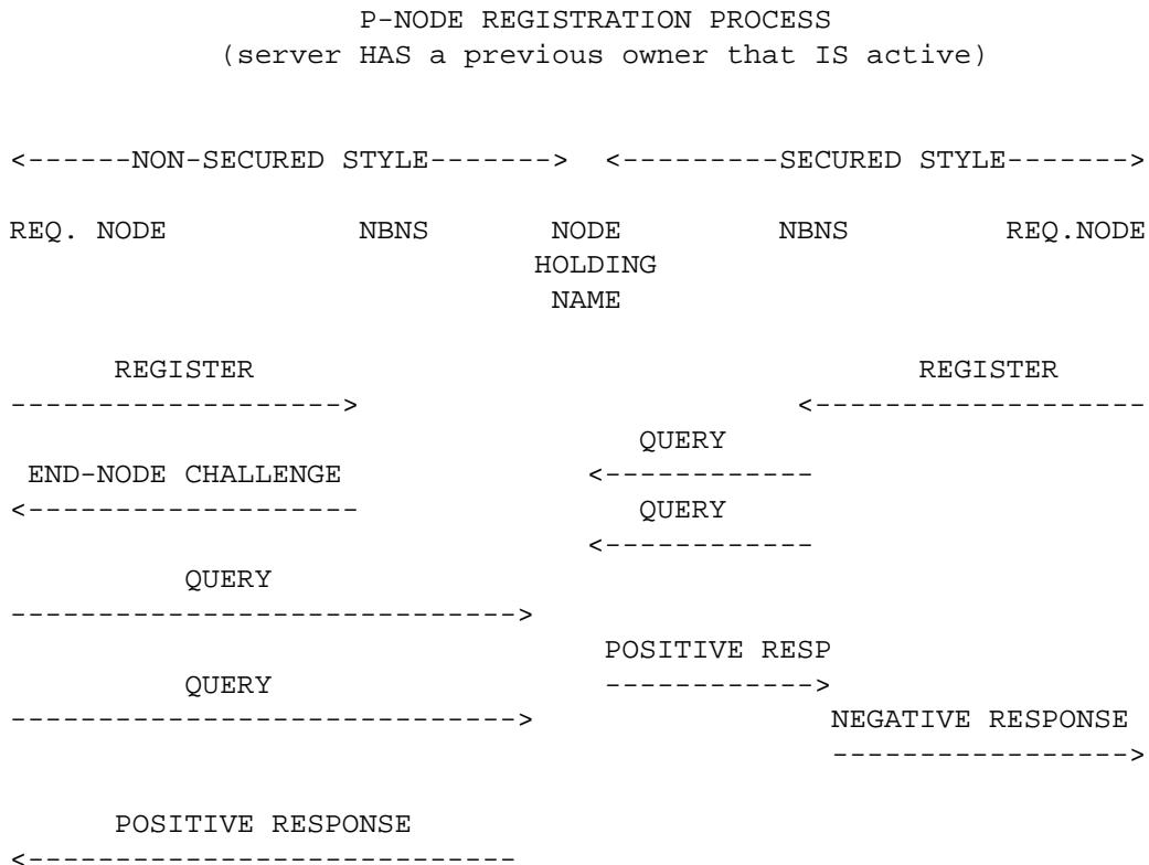
A non-secured NBNS will answer the NAME REGISTRATION REQUEST with a END-NODE CHALLENGE REGISTRATION RESPONSE. This response asks the end-node to issue a challenge transaction against the node indicated in the response. In this case, the prior node will defend against the challenge and the registering end-node will simply drop the registration attempt without further interaction with the NBNS.
