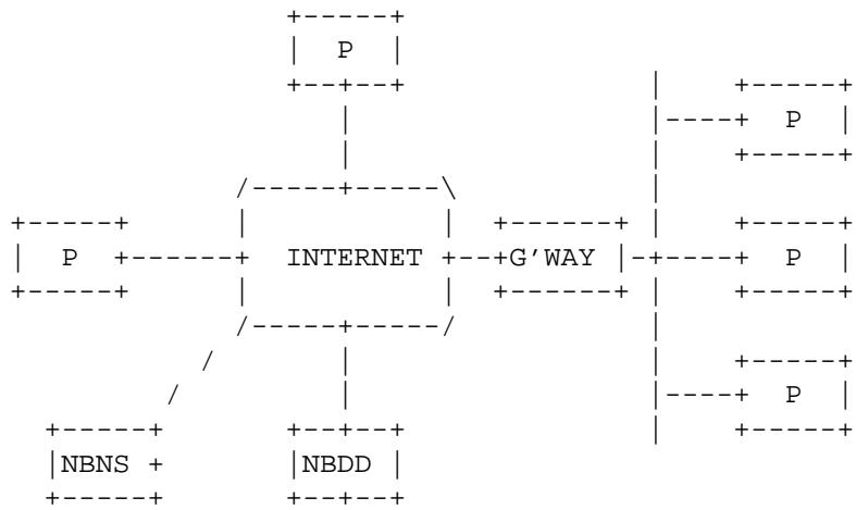
Any P node may be replaced by an M node with no loss of function to any node. However, broadcast activity will be increased in the broadcast area to which the M node is attached.
