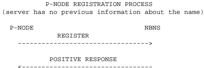
The interaction is rather simple: the end-node sends a NAME REGISTRATION REQUEST, the NBNS responds with a POSITIVE NAME REGISTRATION RESPONSE.
